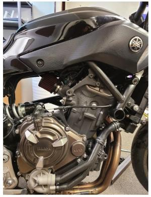
Step 10: install engine mount spacer in the front engine mount frame.
