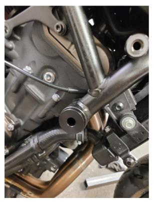
Step 11: With the 12mm and 10mm bolt place them inside the cage, align the cage with the mount points and rear engine bolt and loosely thread the cage into the bike.
