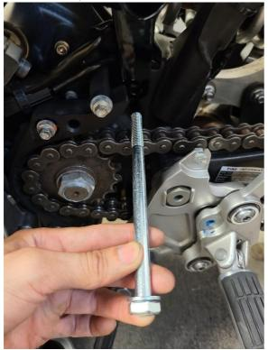
Step 7: Take the top cross bar (longest bar) and remove the assymbled hardware (9/16" or 14mm socket). Go to the right side of the bike and set the cross bar through top section of the frame.
