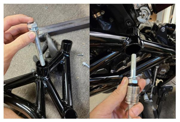
Step 6: Take the 10mm x 1.5 x 150mm place it through the rear plate of the cage and rear engine mount of the motorcycle.
