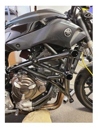
Step 12: Take the lower cross bar and install it between lower cage mount. (RACE RAILS DO NOT HAVE A LOWER CROSS BAR)
