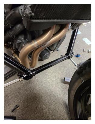
Step 13: Align the top cross bar with the top engine puck mount and thread the 3/8s bolt and washer in.
