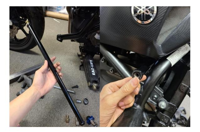
Step 8: take the 3/8s bolt with washer and loosely thread it into the crossbar through the top puck mount.
