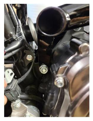
Step 15: Once all mount points are aligned go through each bolt and proceed to torque the bolts to spec
