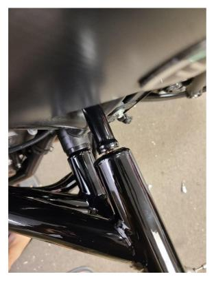
Step 14: Take the 10mm nut and thread it onto the rear engine bolt.
