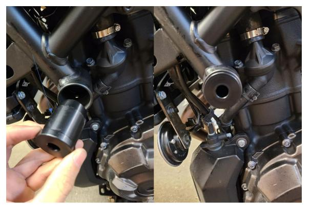
Step 5: With the hard ware provided place the 12mm x 1.25 x 100mm inside the front tube mount and 10mm x 1.25 x 50mm bolt in the center tube mount. Take your cage and line the up with the holes on the bike. Loosely thread the hardware into the bike but do not tighten down yet.
