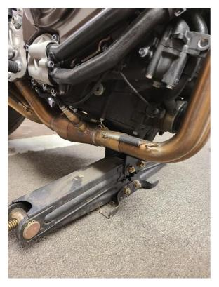
Step 2: Starting on the left side of the motorcycle remove the sprocket cover (5mm Allen key) and shift pedal pivot bolt (6mm Allen key) to access the rear engine bolt. These items will be reinstalled upon completion.
