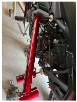
• align the cage with mount points and lightly secure the front mount
