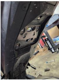
Begin by removing the factory passenger peg and the rear fender eliminator kit from the motorcycle.
