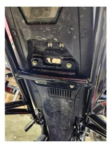
Lift the rear end of the sub cage to fit the rear fender mounting location.
