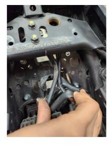
Lightly bolt up the rear with the m6 nuts and bolts through the rear fender and sub cage holes as shown.
