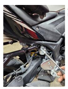
Align the front mount of the sub cage to the front tab on the subframe mount.
