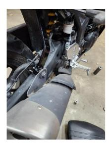
Reinstall the exhaust bolt to the bracket. Then tighten down the M8 nut on the back side of the exhaust bracket.
