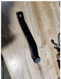
For installing an exhaust bracket remove the OEM grommet and spacer from the rear passenger peg. Install the grommet and spacer into the new bracket provided. Soapy water will help when putting in the grommet.
