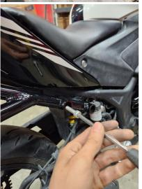
If installing an exhaust bracket. Use the longer M8 bolt provided with the bracket and screw the bolt into the mount location as shown. The exhaust bracket will be place on the back side of the mounting tab as shown on the right figure. Place the M8 nut and lock washer on the back side of the exhaust tab.
