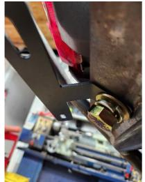
Take the 5/8s bolt and bolt up the rear subcage to the adapter plate.
