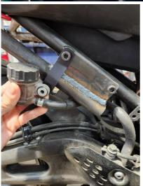
Take the sub cage and lightly bolt up the front tabs to the passenger peg mounts.
