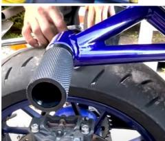
Install the pegs to the sub cage with the hardware provided.
