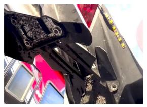
Next Remove the 4 bottom push rivets from underneath the fender.
