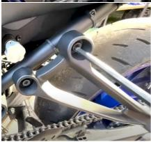
Remove the passenger pegs from both sides of the bike.
