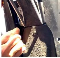
Hold the fairings to the side to access the bolts under neath the fender.
