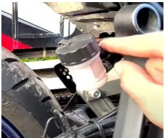
First remove the brake reservoir from the right side passenger pegs. Keep the bracket as it will be reused later on.
