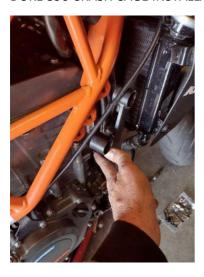
Start by removing the OEM Y brackets from both sides of the bike. The crash cage will replace the OEM bracket. Remove the lower engine mount bolt
