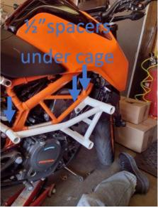
Place 3 of the  $\frac{1}{2}$ " spacer between the frame tab and crash cage plate and rear mount.
