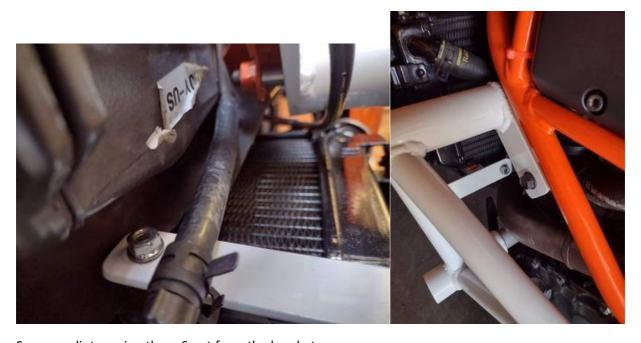
Secure radiator using the m6 nut from the bracket.
