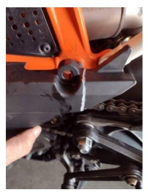
Left side sprocket cover will need to be trimmed for crash cage to fit.
