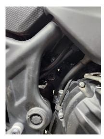
Begin by removing the rear engine bolt.
