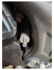
Moving to the left side. Place the 2.5" aluminum spacer on the rear engine bolt.
