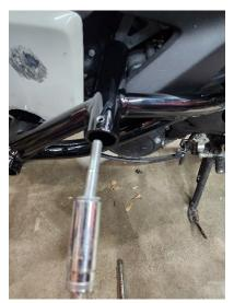
Take the m10 x 60mm and lightly thread to the center engine mount.
