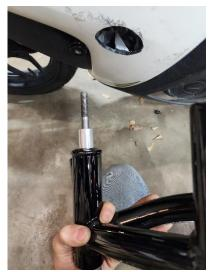
Remove the dust cap off the frame.
