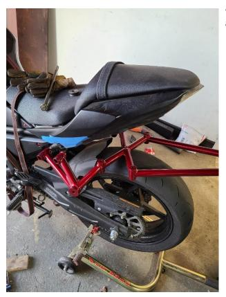
• Remove stock passenger pegs from the frame and place the subcage in place.
