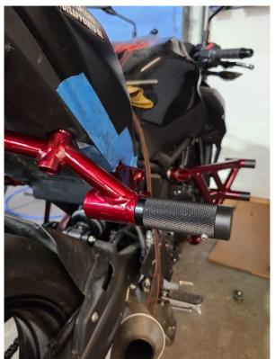
Lift the sub cage up and thread provided the bolt through the tubing mounts.
