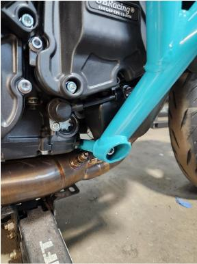
• Place the lower cross bar through the bike and lightly thread the bolt in.
