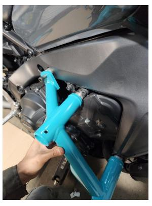
• Lightly thread the bolts into the frame to hold the cage in position. (DO NOT TIGHTEN AT THIS POINT)
