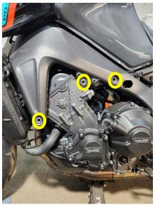
• Going to the left side of the bike remove the three engine bolts circled.
