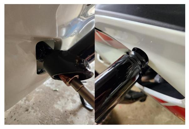
• Once everything is installed proceed to tighten each bolt around the cage.
