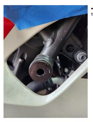
• Insert the engine mount spacer provided into the frame.
