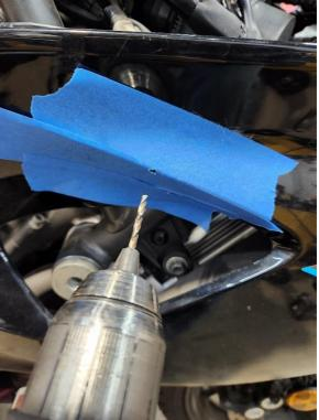
• For the optional top cross bar its best to mask the fairing with painters' tape to lay out the hole for the top cross bar
