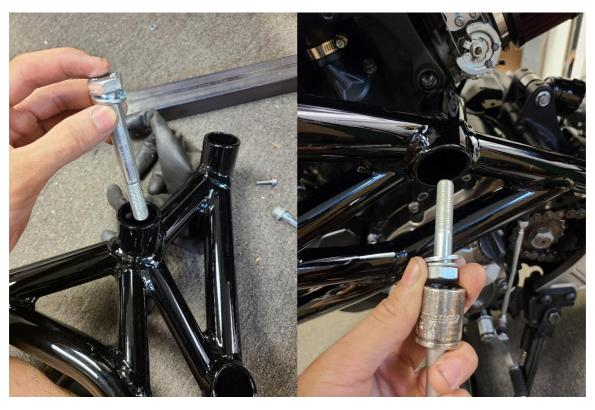
Step 6: Take the  $10 \text{mm} \times 1.5 \times 150 \text{mm}$  place it through the rear plate of the cage and rear engine mount of the motorcycle.
