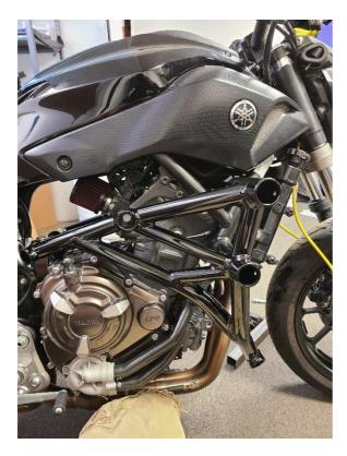
Step 12: Take the lower cross bar and install it between lower cage mount. (RACE RAILS DO NOT HAVE A LOWER CROSS BAR). Newer versions of the cage have a bent lower crossbar.
