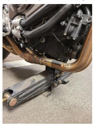
Step 2: Starting on the left side of the motorcycle remove the sprocket cover (5mm Allen key) and shift pedal pivot bolt (6mm Allen key) to access the rear engine bolt. These items will be reinstalled upon completion.
