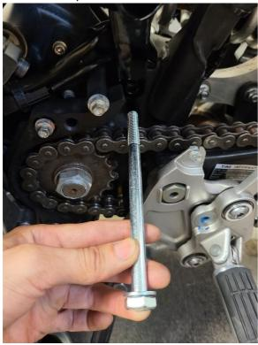
Step 7: Take the top cross bar (longest bar) and remove the assembled hardware (9/16" or 14mm socket). Go to the right side of the bike and set the cross bar through top section of the frame.
