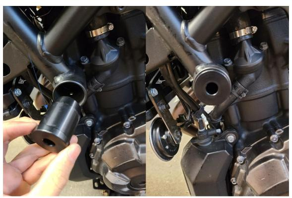
Step 5: With the hardware provided place the  $12mm \times 1.25 \times 100mm$  inside the front tube mount and  $10mm \times 1.25 \times 50mm$  bolt in the center tube mount. Take your cage and line the up with the holes on the bike. Loosely thread the hardware into the bike but do not tighten down yet.
