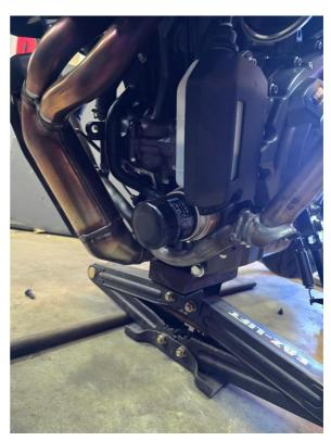
Step 13: Align the top cross bar with the top engine puck mount and thread the 3/8s bolt and washer in.
