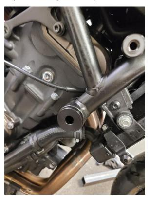
Step 11: With the 12mm and 10mm bolt place them inside the cage, align the cage with the mount points and rear engine bolt and loosely thread the cage into the bike.
