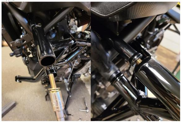
Step 9: Now on the right side of the bike remove the front engine mount and middle engine bolt.
