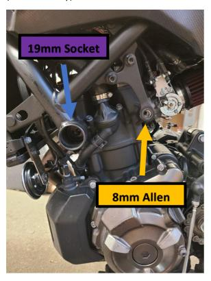
Step 4: Take your engine mount spacer and place it inside the front frame mount
